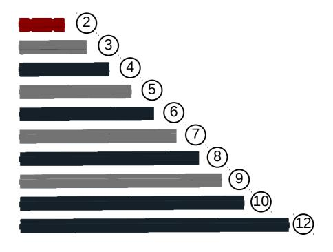
Axles will rotate and slide in beam holes unless constrained
