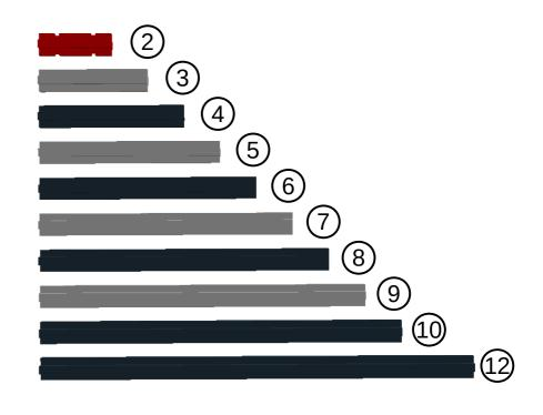
Axles will rotate and slide in beam holes unless constrained
