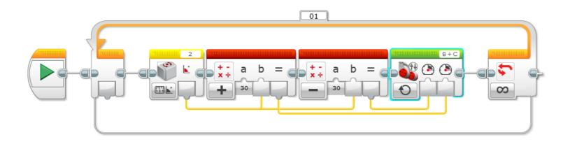
To follow a gyro angle other than zero, subtract the desired heading from the gyro angle:
