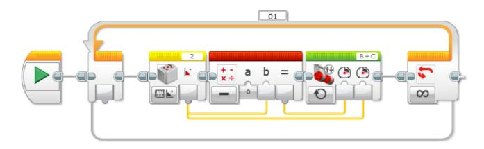
Let's add a math block to the loop that adds the gyro angle to zero:
