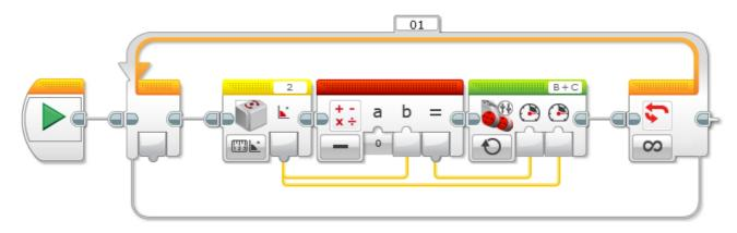
The gyro sensor block reads an angle
