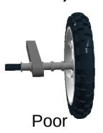
Axles do better when supported by at least two beams. Beams on both sides of wheel are best.
