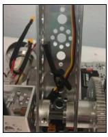
On a competition robot the connectors for the motor cables should be secured to the motors, e.g., using electrical tape. This ensures that the connectors do not fall off during competition.
